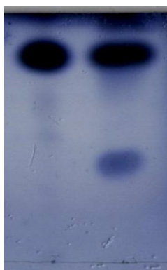
Figure 2. TLC Analysis of D-galactofuranosylation products of D,L- \alpha -tocopherol. Start 1, D,L- \alpha -tocopherol; start 2, reaction products. Migration, SS II. Visualisation, mostain.
